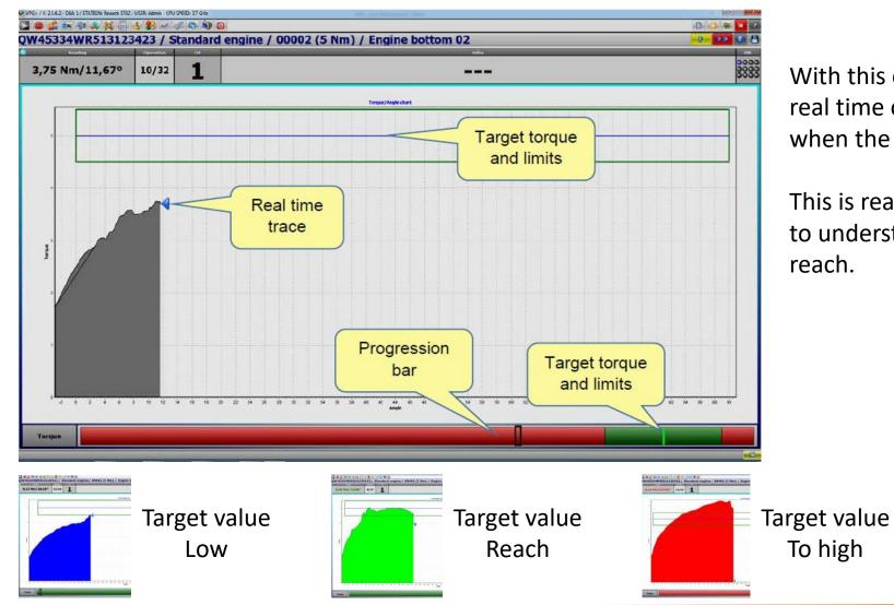
With this option, the operator can see the trace in real time on the computer screen and stop to tight when the trace change from Blue to Green.
